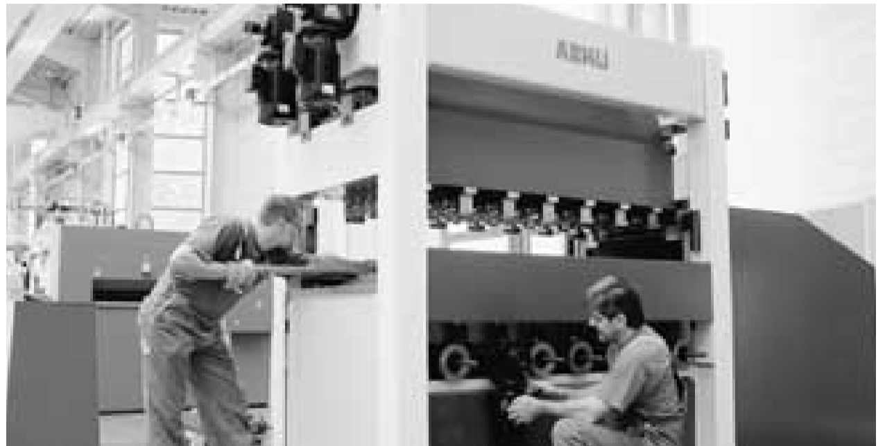
One Arku 6-high leveler during final assembly
