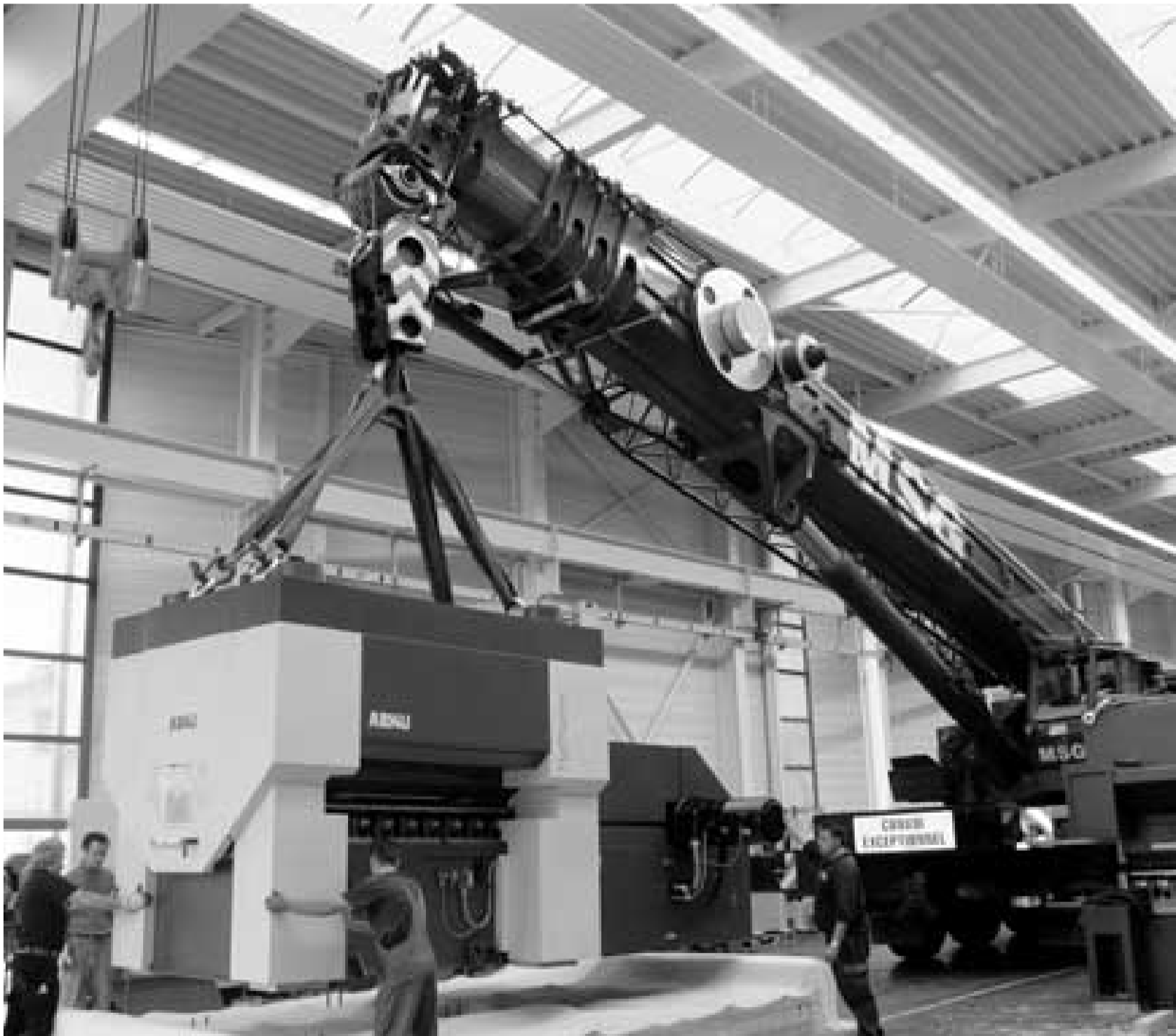
One FlatMaster 80 for sheet metal parts up to 20 mm thickness on its way to Mexico
