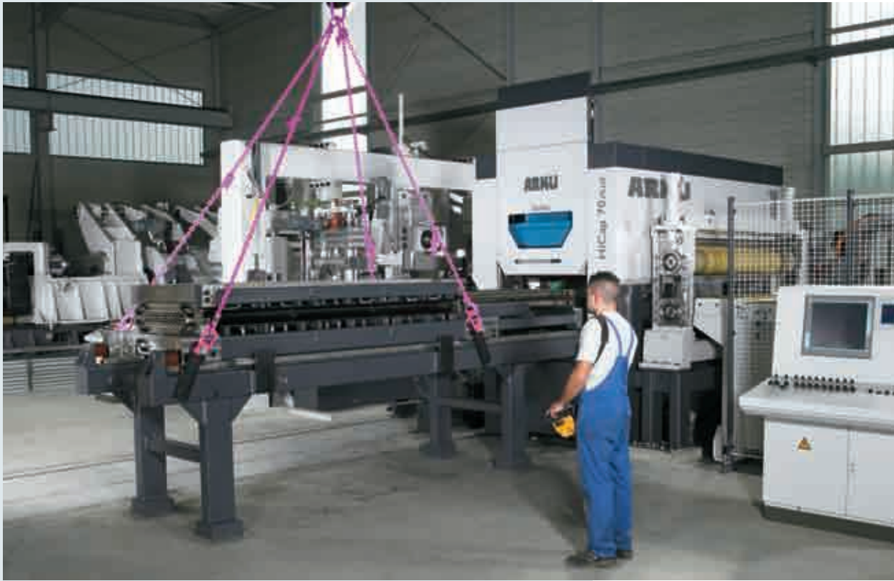
ARKU HiCap® PLUS – equipped with a cassette change system for varying roller diameters
